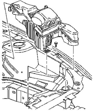
1. Remove the air cleaner housing assembly.
