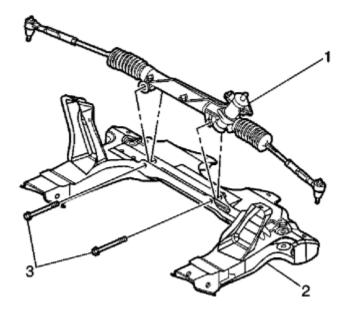
14. Remove the power steering gear mounting bolts.15. Remove the frame.
